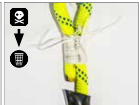
Termination with torn safety stitching
