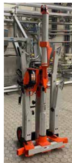
TwinSleeve davit Trolley for easy transport.
