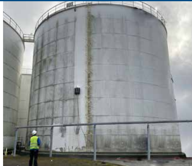
Tank-cleaning robot on the outer shell—protected by two LA33/85 that arrest the unit if the primary tether/cabling fails.
