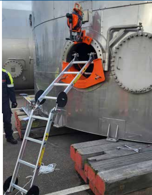
HangingLadder® shown in a hinged position for insertion through the manhole; once fully inserted, it hangs vertically and is ready for use.
