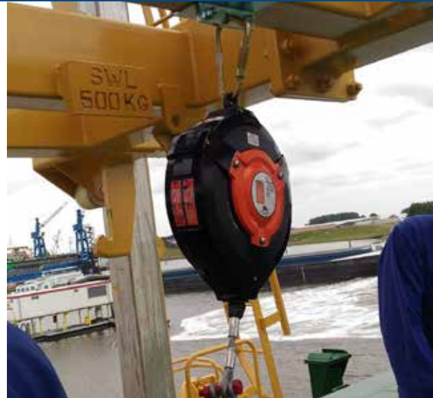
Shipboard installation of the LA15/500 load arrestor—engages to stop the load if the primary support fails.
