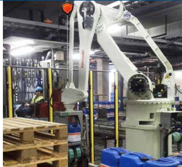
Industrial palletizing with overhead LA15/300—stops the suspended load on primary failure (300 kg max).
