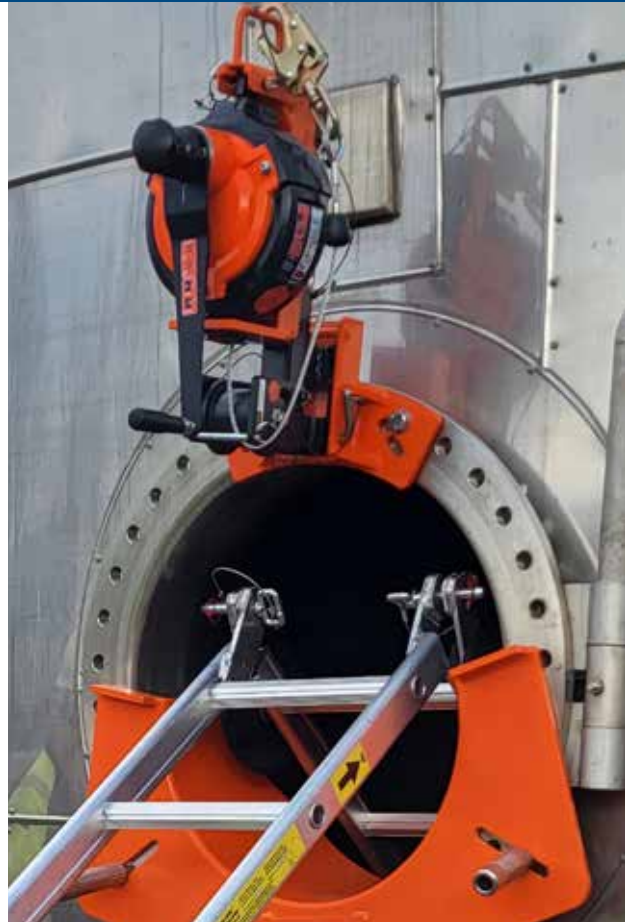
Combination of FlangeClamp, FAB15R, RescueSlide and HangingLadder. (Photo showing feeding HangingLadder system in vessel through horizontal manhole).
